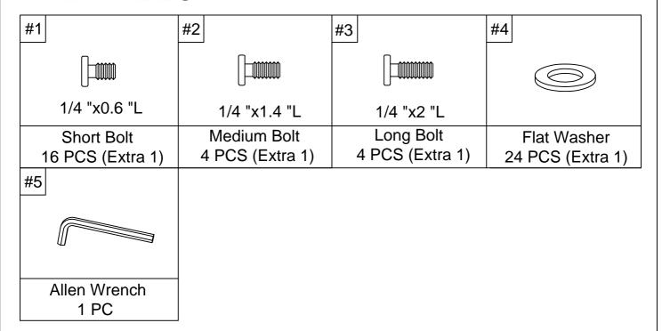
Step1: Lay seat frame (part D) down on a soft flat surface, such as carpet, as shown below. Attach left leg (part B) and right leg (part C) to seat frame (part D) using medium bolts (part #2), flat washers (part #4) and allen wrench (part #5).
