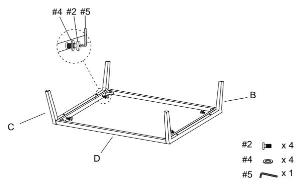
Step 2: Attach left leg (part B) and right leg (part C) to seat panel (part A) using long bolts (part #3), flat washers (part #4) and allen wrench (part #5).
